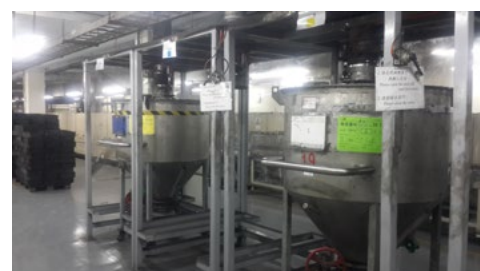
Changing the way of inputting the raw material into the production line from manual to piping
